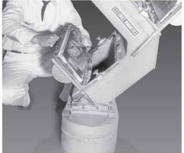
This magnetic hump separator is one of the most reliable safety devices in a distillery. The separator is so efficient not even a wayward thumbtack gets by.
