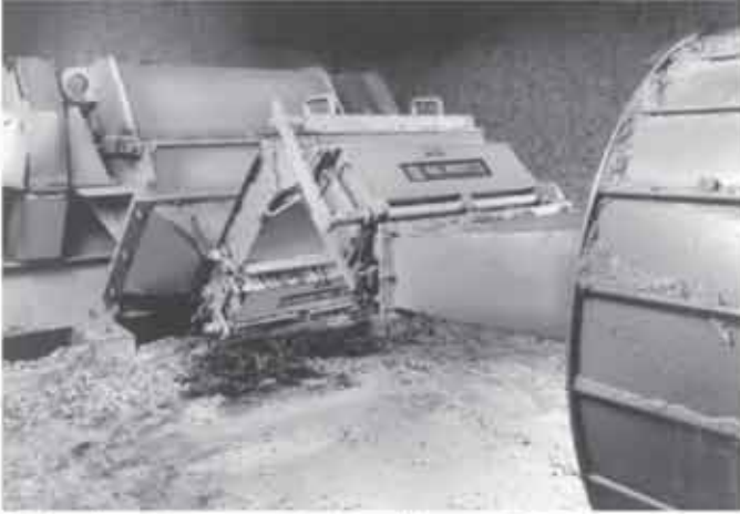
This pallet grinding application utilizes an Eriez Hump to separate steel nails from wood chips.
