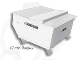
The standard chute separator is equipped with support legs designed for installation in a 50° chute as shown, but can be easily modified for greater or lesser slopes as required. An access door built into the chute-work below the magnet is necessary for the periodic removal of accumulated tramp iron. The cooling oil fill and drain connections are readily accessible with the magnet in position.
