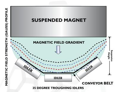
Typical magnetic field configuration of an electromagnet suspended over a conveyor belt. The magnetic field extends outward from the center of the magnet. The magnetic field is strongest at the center and diminishes towards the edges.
