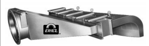
This close-up of an Eriez Flocculator Magnet and the photo at right below show how the flocculator can be installed easily and quickly in the inlet pipe to the clarifier. Its design forces water to be spread out over a large area. Magnetic flocculation requires only split-second exposure to magnetic flux generated by the permanent magnets on top and bottom. Maintenance costs are virtually nil.
