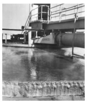
Eriez Flocculator Magnet installation at a large steel plant is shown above. Magnetic flocculation reduced ferrous solids in overflow from 600 parts per million to as low as 40 parts per million.
