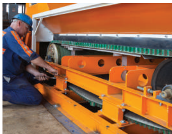
Loosen Support Blocks
